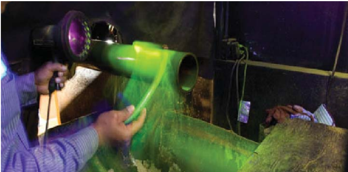
picture 3: Special-End-Area Inspection
