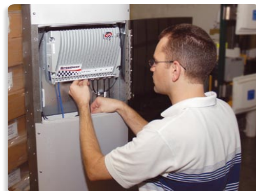
A technician at ADT's EPCglobal-accredited RFID Performance Test Center in Boca Raton, Florida, makes the final connections on an Impinj UHF Gen 2 Speedway™ reader.
